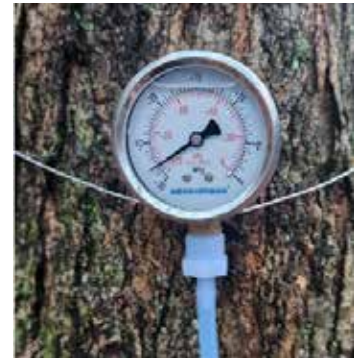
Getting high levels of natural vacuum on 3/16" lines.
